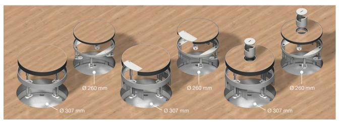
Round cartridge unit with hem made of stainless steel with an external diameter of 307 mm as a dummy cartridge unit, cable outlet cartridge unit and tube cartridge unit for the installation into screed and hollow floors. For 12/30 mm parquet and stone covers and linoleum in combination with rigid foam lid insert. Can be levelled from 100 to 155 mm.
